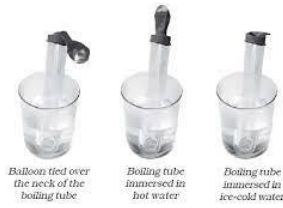
Fig. 8.6 The shape of the balloon in hot and cold water
